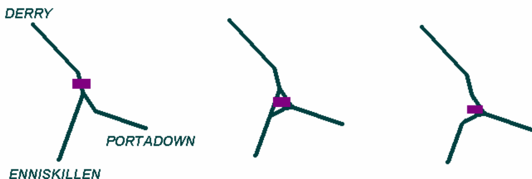
Fig 9 – The original Omagh station was located just north of the junction with the Enniskillen and Portadown lines (left). Under NINE, the station could be re-built in a triangular format, allowing through running of services in all directions (centre). Alternatively, the junction could be re-built facing Portadown, with passengers travelling from Enniskillen to Londonderry changing at the station. If the station was located in the “vee” of the junction, cross-platform interchange would be possible. Also, the station would not have to be located at the original site.
