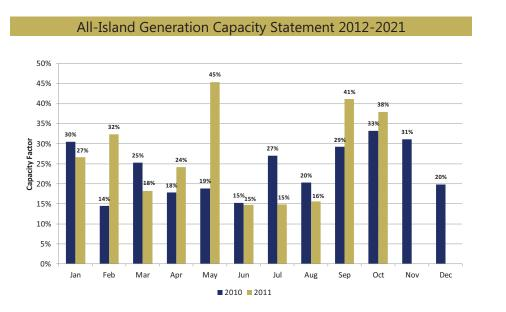
Figure 3-8 Monthly wind capacity factors in Northern Ireland for 2010 and 2011.
