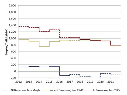
Figure 4-6 The effect of losing the benefit of the 2 undersea interconnectors from the Base Cases
