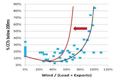
Figure 5-3 Percentage of contingencies causing Critical Clearance Times (CCT) lower than 200ms vs SNSP ('Facilitation of Renewables', 2010). Potential impact (red curve) on transient stability if wind farms' dynamic reactive power capability is not clarified in the Grid Code
