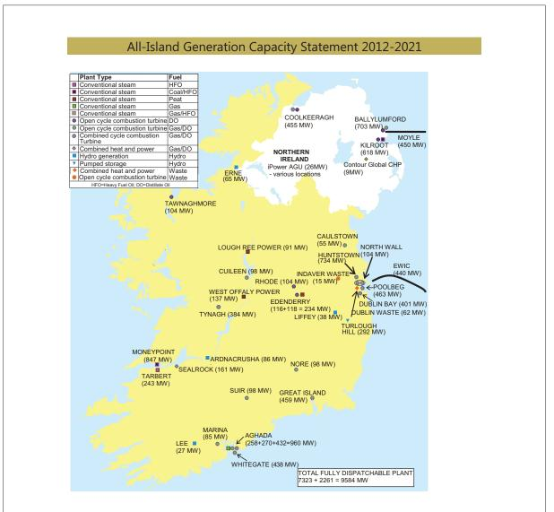
Figure 3-1 Fully dispatchable plant installed in 2018, at exported capacities. All figures shown are maximum export capacities – generators may often operate at a lower export capacity.
